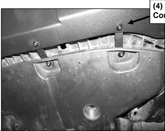
(Fig 23) Attach Splash Guard Support Brackets to back of Bumper (also see Fig 8)
