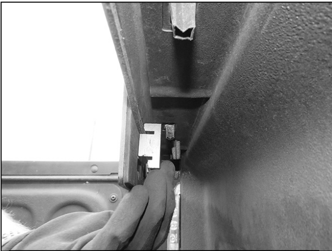
(Fig 8) Check back of lip on bed for clearance and to determine installation procedure
