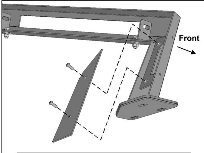
(Fig 1) Remove cover plates from Light Bar
