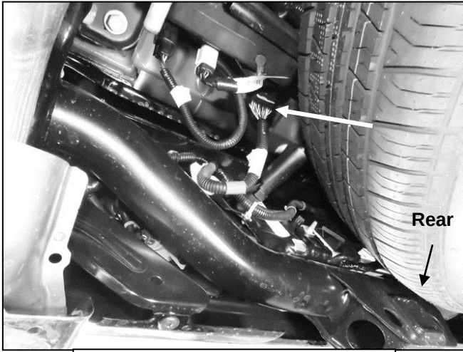
(Fig 3) Unplug all wire harnesses leading to the Bumper
