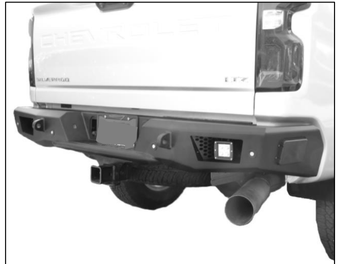
(Fig 26) Adjust Bumper and tighten hardware (lights not included)
