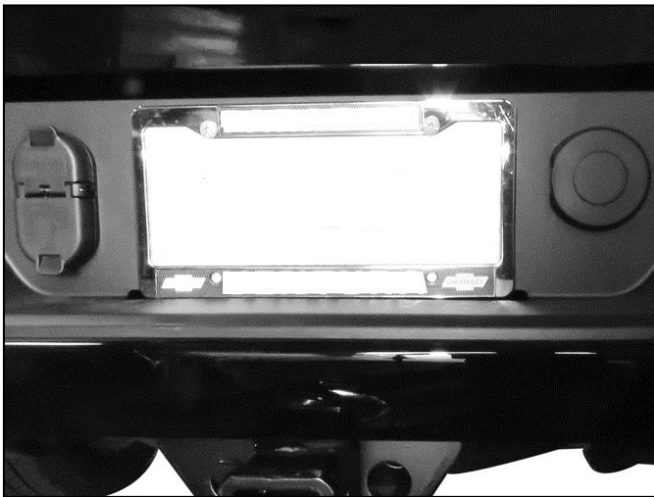
(Fig 1) Remove the license plate from the rear bumper
