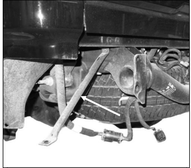
(Fig 7) Remove the outer bumper supports from both sides of the frame (driver side shown)
