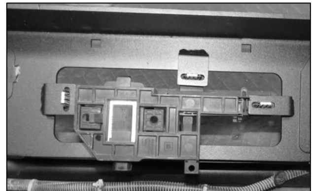
(Fig 17) Attach remote antenna assembly installed on the Bumper
