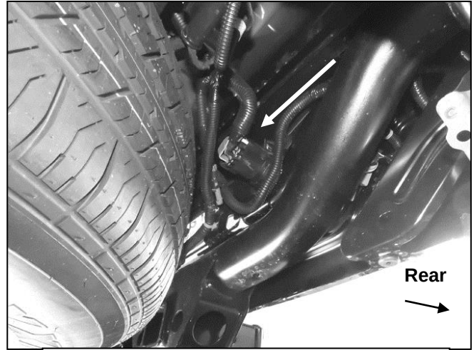
(Fig 4) Disconnect the trailer plug Note: Some vehicles have additional wires on the trailer plug that must be disconnected
