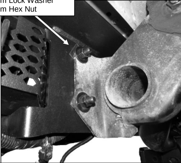
(Fig 25) Attach Bumper to frame (driver side shown)
