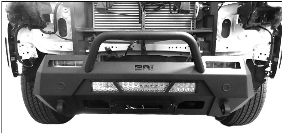
(Fig 61) Center bumper on vehicle and tighten hardware
