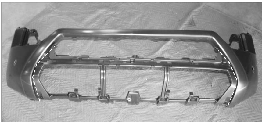
(Fig 36) Trim lower section of front clip under guidelines. Bumper disassembled for illustrative purposes only
