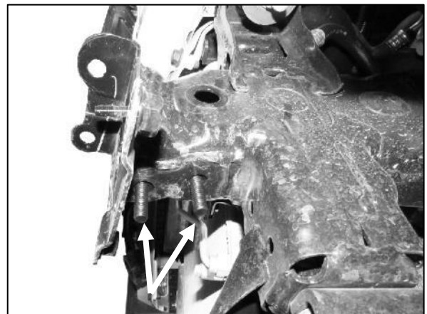
(Fig 42) Ensure both bolts go through the bottom slots of the frame.
