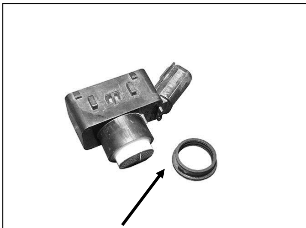
(Fig 51) Remove rubber seal from end of sensors
