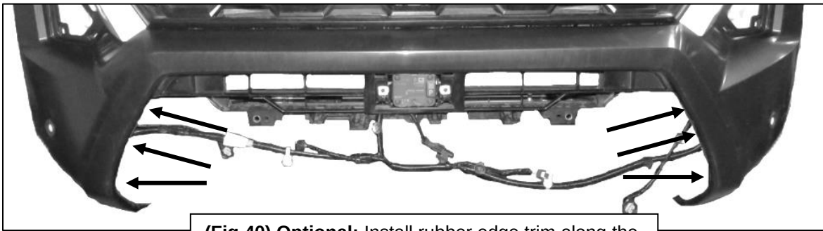
(Fig 40) Optional: Install rubber edge trim along the sides of the factory plastic front fascia
