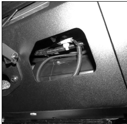
(Fig 67) Reach through the lower openings on each side of the Front Bumper Assembly and plug in the fog lights and front parking sensors using the Parking Sensor Extension Harnesses (if equipped)
