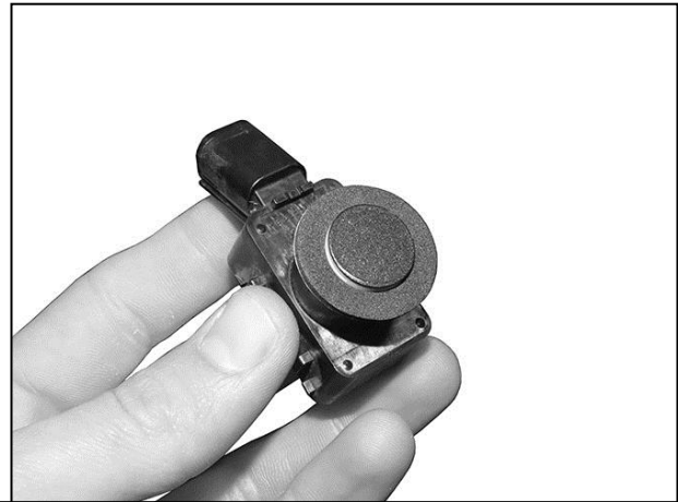
(Fig 52) Apply Adhesive Foam ring to end of sensors
