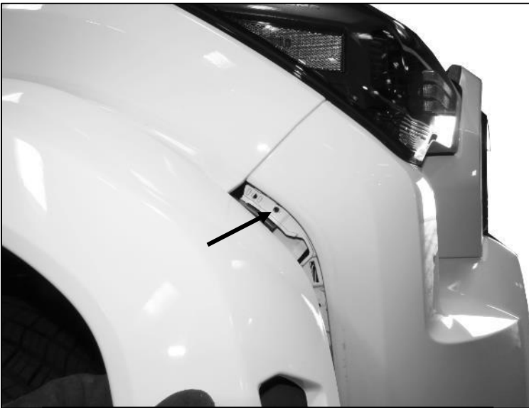
(Fig 3) Remove screw attached to side of front clip behind fender flare.
