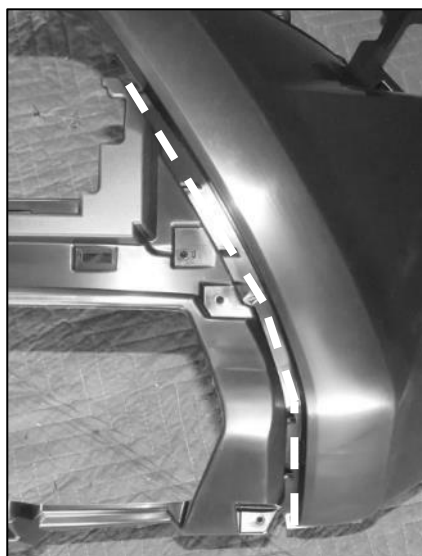
(Fig 37) Cut along the edge on the side of the front clip
