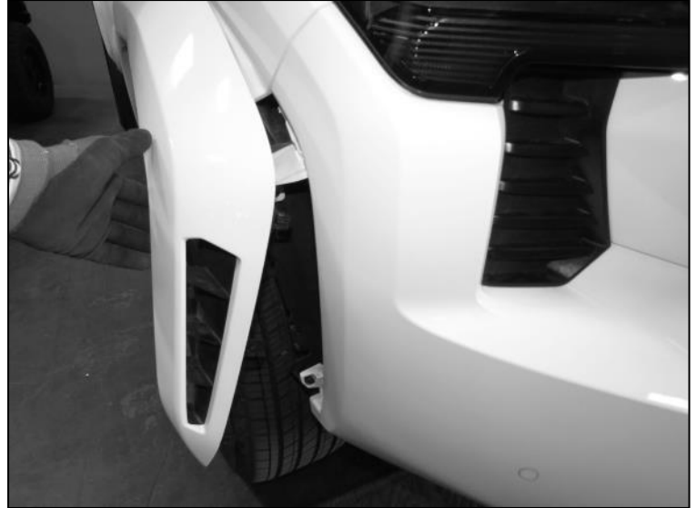
(Fig 2) With a pry tool, carefully pull the fender flare outwards to release it from the side. Repeat on Driver side.
