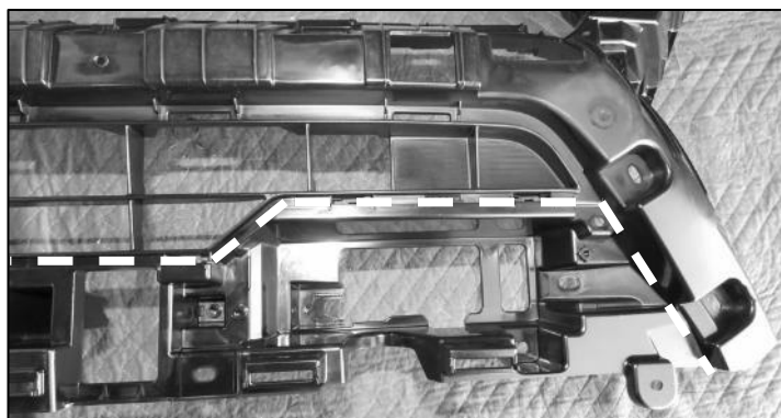
(Fig 33) Cut along the edge on the side and under the grille opening
