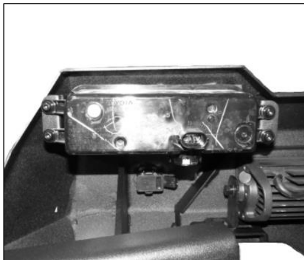
(Fig 56) Factory Fog Light installed onto Fog Light Mounting Tabs (Driver side shown).
