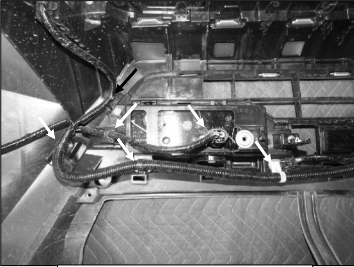
(Fig 28) On Left fog light area, unfasten indicated clips and unplug fog light. Repeat for Right fog light.
