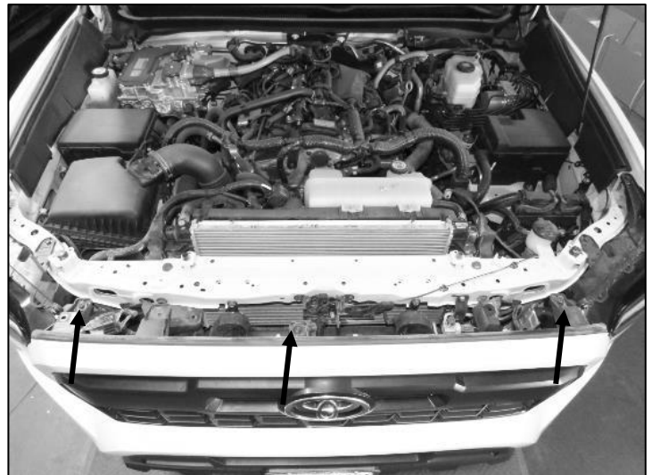
(Fig 12) After removing plastic covers and air intake, remove three bolts holding the upper clip.
