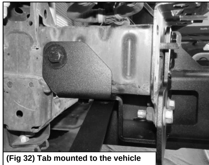
(Fig 31) Attach tab on Winch Tray to side of frame
