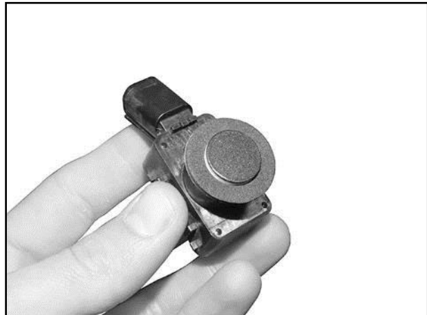
(Fig 52) Apply Foam Seals to end of sensors
