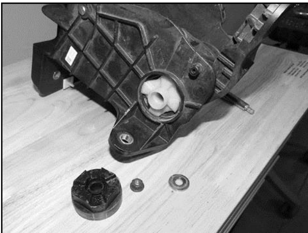
(Fig 15) Remove outer covers and inner drive from both sides
