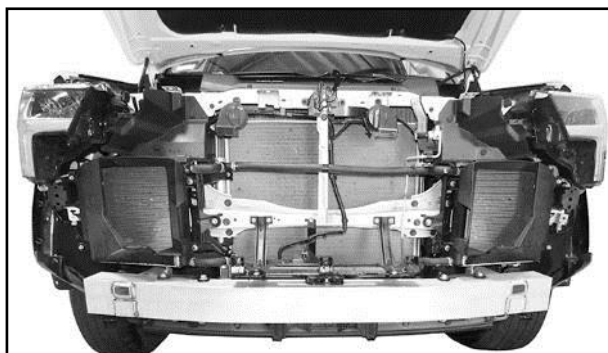
(Fig 6) Unplug all wiring harnesses leading to front bumper (passenger/right side pictured)
