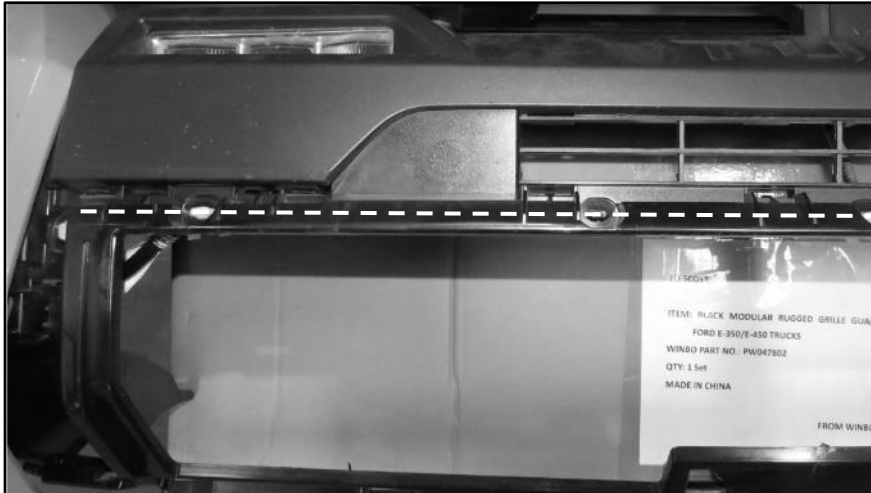
(Fig 43) Begin trimming the center plastic as depicted, make sure to NOT cut off the mount tabs under the fog lights as they secure the top plastic panel
