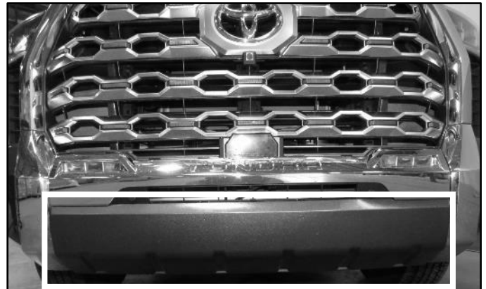
(Fig 40) Lower cover should've been removed from earlier steps (Refer to fig 4)
