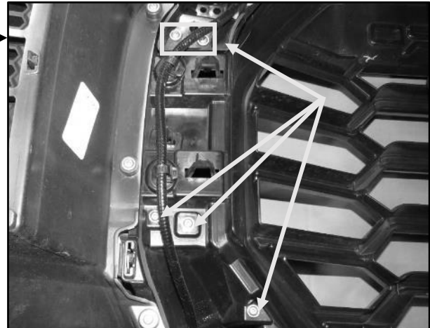
(Fig 38) Three screws need to be removed on the inside of the factory bumper on each side before the painted pieces can be removed
