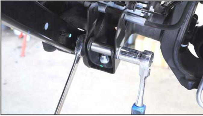
**25. Tighten the lower shock bolt using an 18mm socket and wrench. Torque to 55ft/lbs.**
