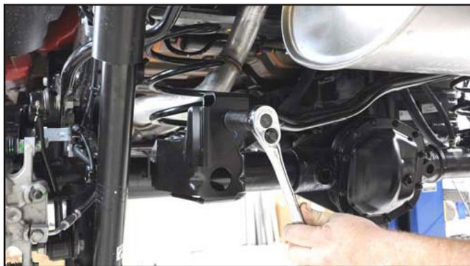
**4. Use an 18mm socket and wrench to remove the lower shock mounting hardware.** Save for reuse.
