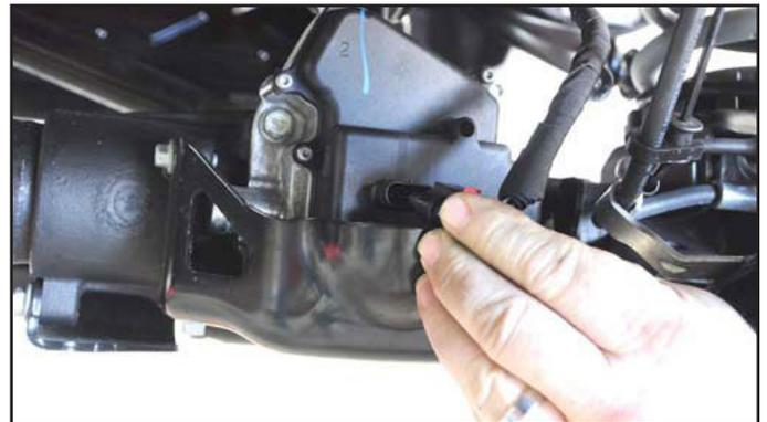
**32. Attach the sway bar links, to the axle, using the factory hardware and an 18mm socket and wrench. Torque to 55t/lbs.**
