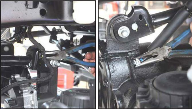
11. Loosen the upper control arms using an 18mm wrench.
