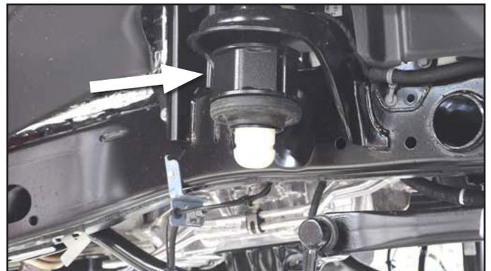
17. Re-install the coil spring.
