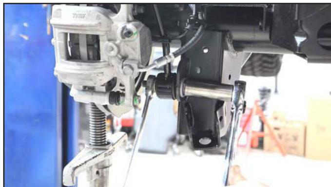
**6. Lower the axle and remove the coil spring and coil spring isolator.**
