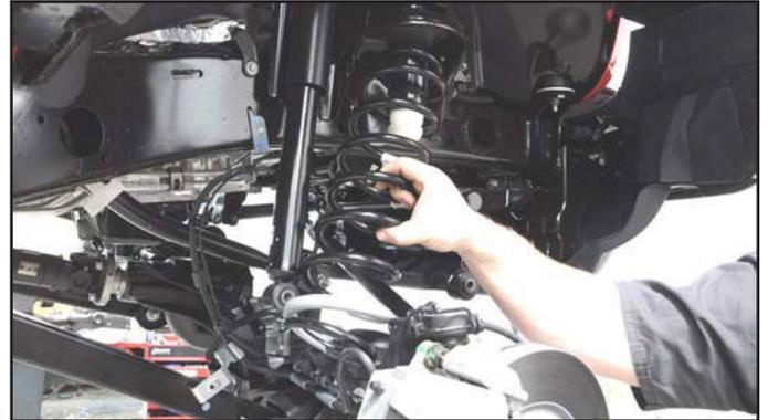
15. Use a 10mm wrench to disconnect the brake line bracket from the lower coil spring mount. Retain hardware for reuse.
