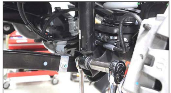
9. Use a 15mm wrench to remove the brake line bracket from the lower control arm. Retain the OE hardware for re-use.
