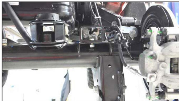
**8. Use a 9/16" wrench and socket to torque the hardware to 30ft/lbs.**
