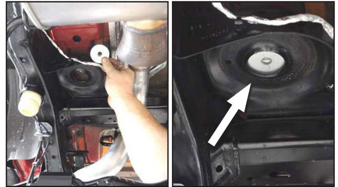
13. Install the supplied rear coil spacer, using the supplied 1/2" x 2.5" bolt. Tighten using a 3/4" socket. Torque to 65ft/lbs.
