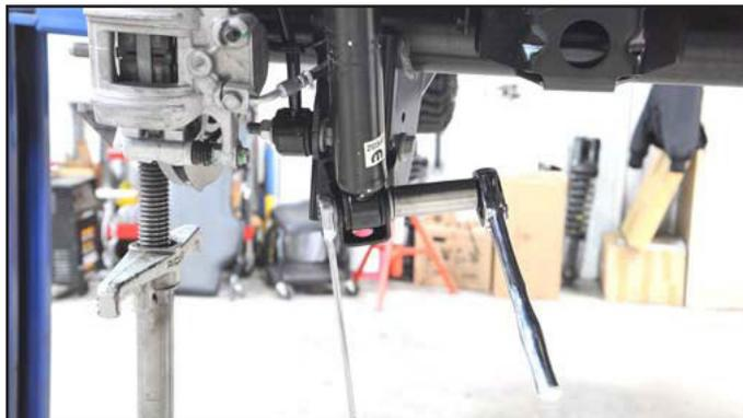
**5. Use an 18mm socket and wrench to remove the lower sway bar link hardware.**
