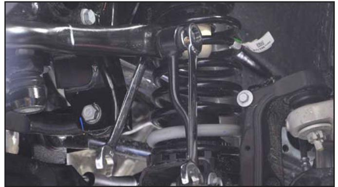
**29. Clip the wiring harness into the upper control arm.**
