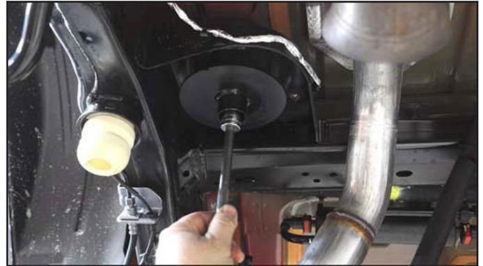
14. Install the coil spring isolator and coil spring.
