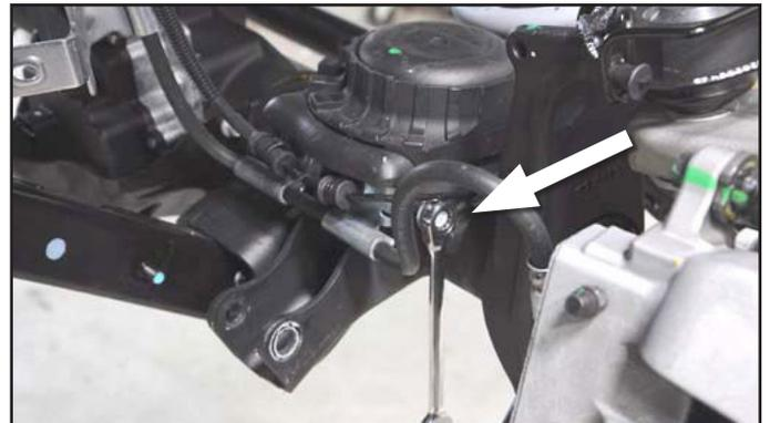
16. Install the supplied spring spacer with coil spring isolator under the spacer.
