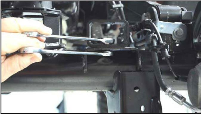
9. Use a 6mm hex key and an 18mm wrench to remove the sway bar link from the sway bar.
