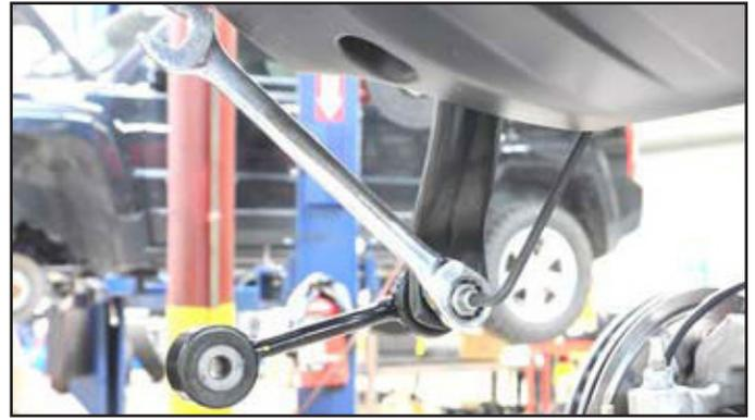
**28. Install the new supplied bent sway link using the supplied 12mm x 65mm bolt, 1/2" washers, and lock nut. Torque to 55ft/lbs.**
