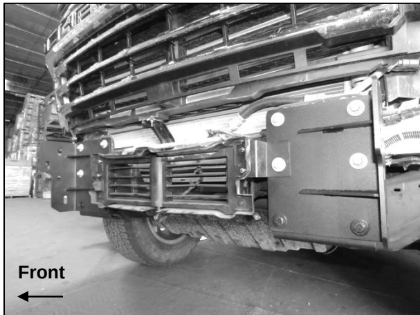
(Fig 20) Attach Relocation Brackets to front of Frame Brackets. Attach shutter assembly, (if equipped), to front of Relocation Brackets
