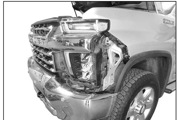
(Fig 4) Remove plastic fascia from top of bumper
