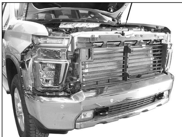
(Fig 7) Grille and fascia removed
