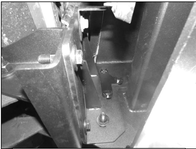
(Fig 33) Driver/Left side of Bumper attached to Mounting Bracket. (Inner side)
