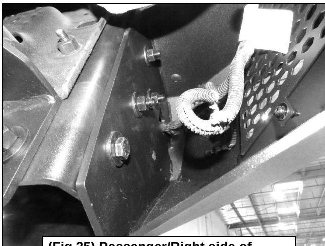
(Fig 35) Passenger/Right side of Bumper attached to Bumper Bracket. Sensor installation also pictured
