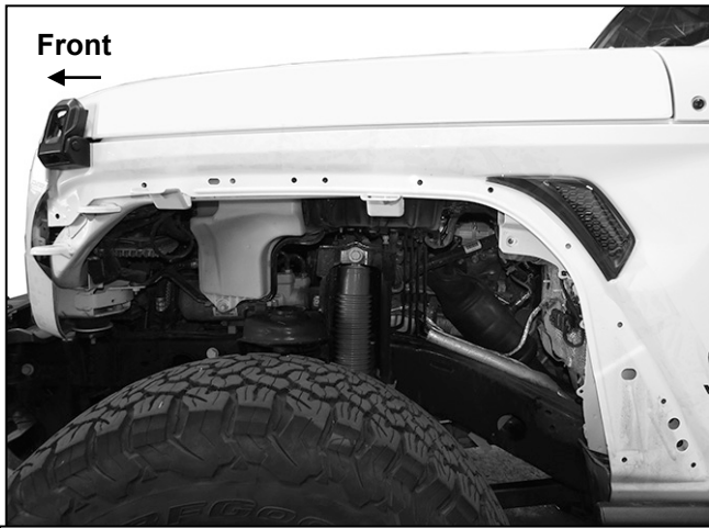
(Fig 3) Firmly pull fender straight out from vehicle
