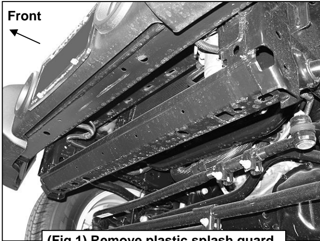
(Fig 1) Remove plastic splash guard or skid plate from bottom of bumper
