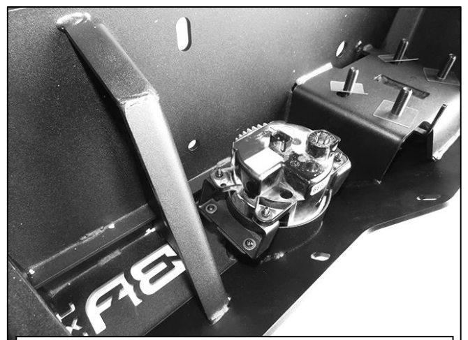
(Fig 10) Factory fog light attached to the back of the Bumper (4 pin fog light mounting shown)
