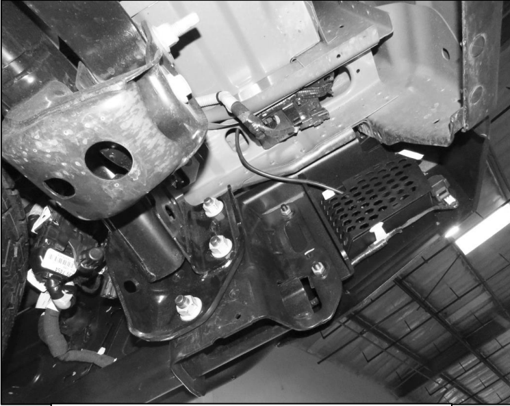
(Fig 26) Plug in main wire harnesses and all other harnesses to vehicle. Ensure bumper is level before fully tightening all hardware.
