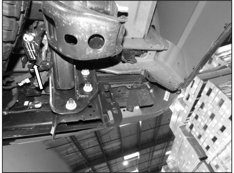
(Fig 2) Unplug all wiring harnesses on Driver Side leading to the rear bumper and move harnesses away from bumper.
