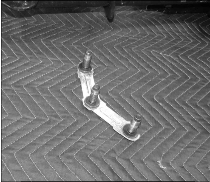
(Fig 9) Factory triple bolt plate removed from assembly. We will reuse on Ambush Rear Bumper.
