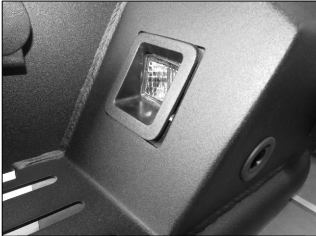
(Fig 14) Depending on model year (2021-2023 or 2024+), install license plate light brackets. Install factory license plate lights into the side wall slots on the bumper
