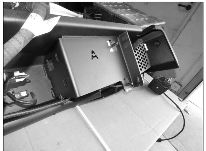
(Fig 21) Before: Long 10mm Double Bolt Plate in position with plastic retainers.
