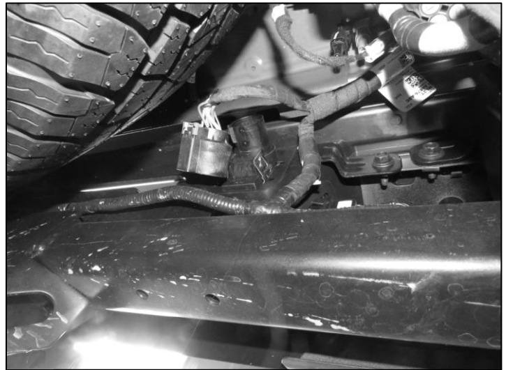
(Fig 4) Unplug trailer harness from trailer plug behind the bumper.
