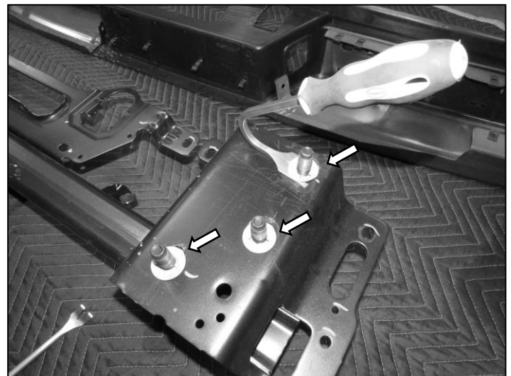
(Fig 8) Remove retaining clip on factory triple bolt plate to remove from hitch. If factory triple bolt plate is attached to bumper instead, remove from bumper.
