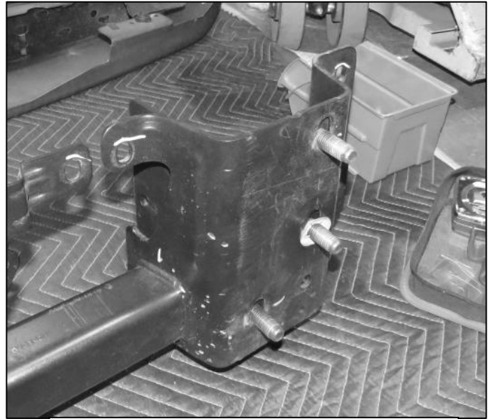
(Fig 19) Using factory retaining clips to keep the factory triple bolt plates in place
