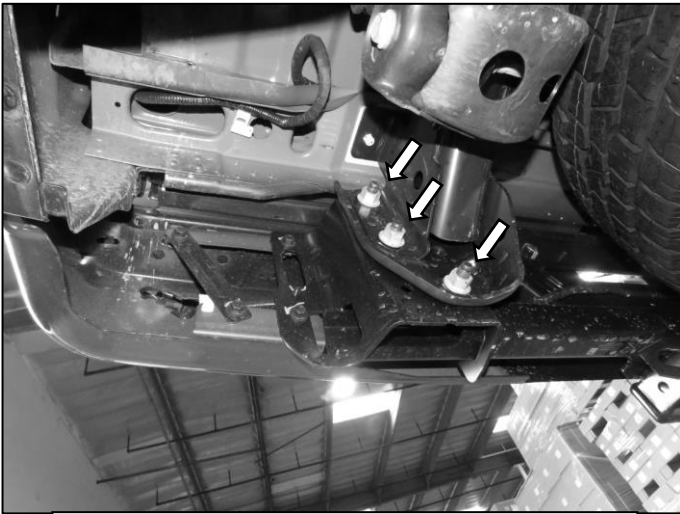
(Fig 3) Remove the hardware attaching the bumper assembly to the end of the frame for both sides. Assistance is required to hold the bumper in place during hardware removal.
