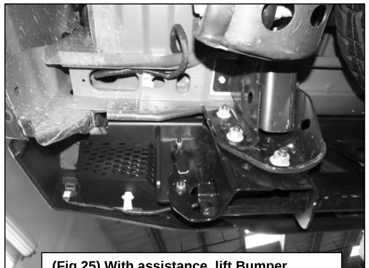
(Fig 25) With assistance, lift Bumper assembly and align it with the end of vehicle frame. Slot in the Factory Triple Bolt Plate into the frame slots and secure with Factory Nuts.
