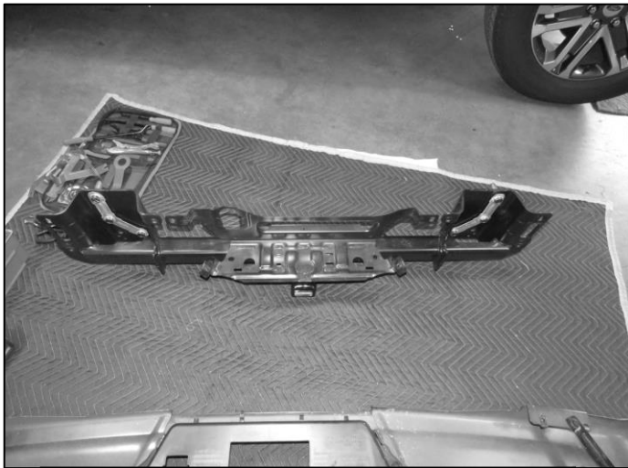
(Fig 7) On models with "HD" tow package with integrated hitch, remove hitch/bracket assembly from back of factory bumper.
