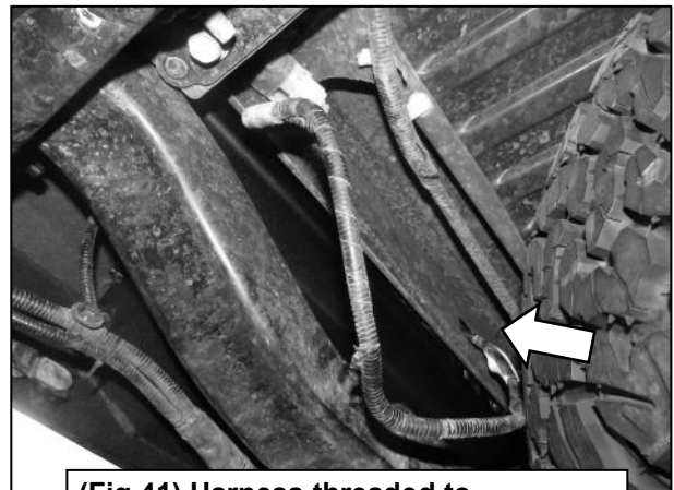
(Fig 41) Harness threaded to underside using spare tire access hole
