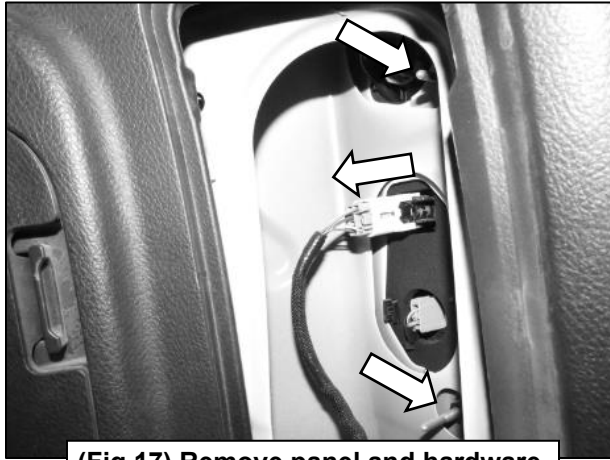
(Fig 17) Remove panel and hardware to remove Passenger/Right rear light
