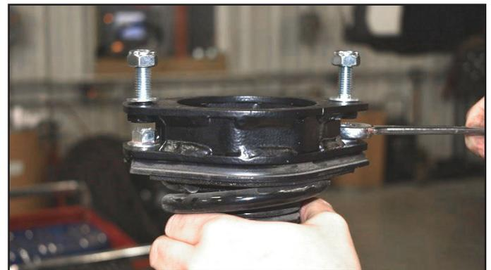
**33. Install the completed strut assembly to the car using the provided M10 flange nuts. Do not tighten at this time. A helper is recommended.**
