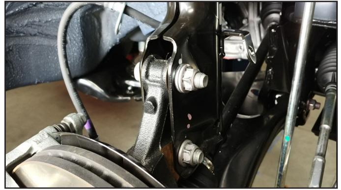
9. **With the lower control arm supported by the jack stand,** release the knuckle from the strut body and let it, along with the lower control arm, hang out of the way. Be careful not to over-extend the CV axle, brake line or ABS harness (adjust the jack if necessary).
