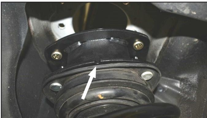
Use the provided M10 hardware with flange nuts to attach the strut assembly to the strut tower. Leave the fasteners loose, to aid in installation of the knuckle.
