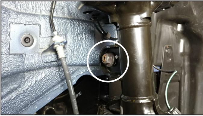
6. **Disconnect the brake line bracket from the strut body** (DO NOT disconnect the brake lines themselves). Let the brake line and bracket hang out of the way.
