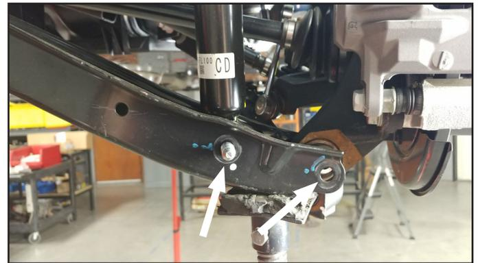
**31. Remove the strut assembly from the vehicle and let the control arm hang.**
