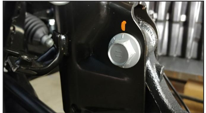
**16. Re-install the brake line bracket to the strut** body, but with the bracket rotated as shown in the photo. Originally the brake line was attached from the bottom upwards to the strut, now it will be mounted to the top of the strut body using the factory hardware.
