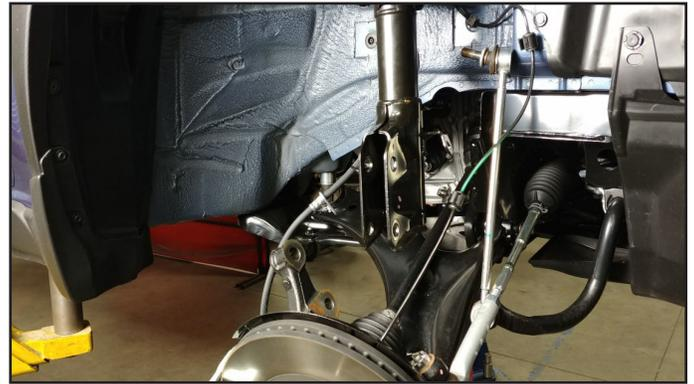
10. **Remove the three (3) nuts that attach the upper end of the strut to the strut tower** (accessed from the engine bay, as the hood should already be propped open). Do not let the strut fall as you remove the last bolt. It may be helpful to have a friend hold up strut as the bolts are removed. Carefully lower the strut and remove it from the vehicle.
