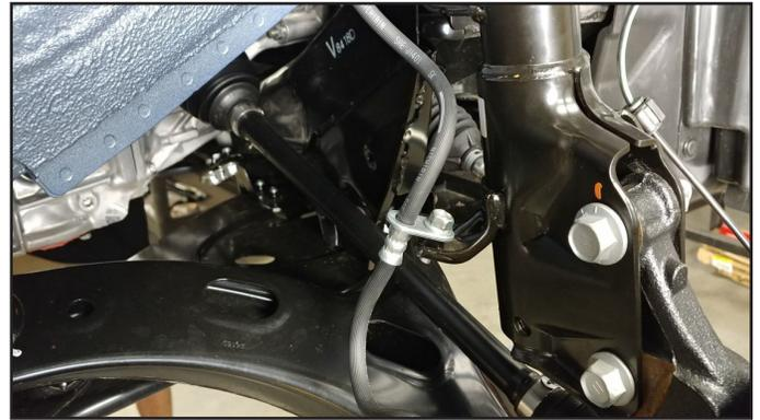
**15. The cam bolt's head flange has hash marks that** correspond to a notch on the strut body. Rotate the cam bolt until the hashes are facing the inside of the vehicle, and align the last hash mark with the notch. This will set camber to maximum negative. Torque both bolts to 95 ft-lbs.
