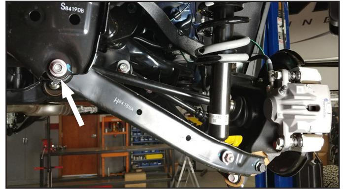
**30. Support the strut and lower control arm, remove the lower strut and knuckle bolts. Lower the control arm down, while holding the strut. Remove the strut from the vehicle. A helper is recommended to hold the strut from falling.**
