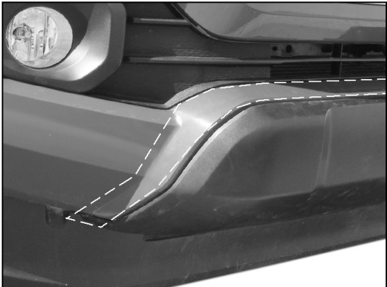
(Fig 4) Cover the sides of the bumper with removable tape (masking tape for example)
