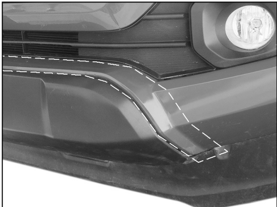
(Fig 5) Cover the sides of the bumper with removable tape (masking tape for example)
