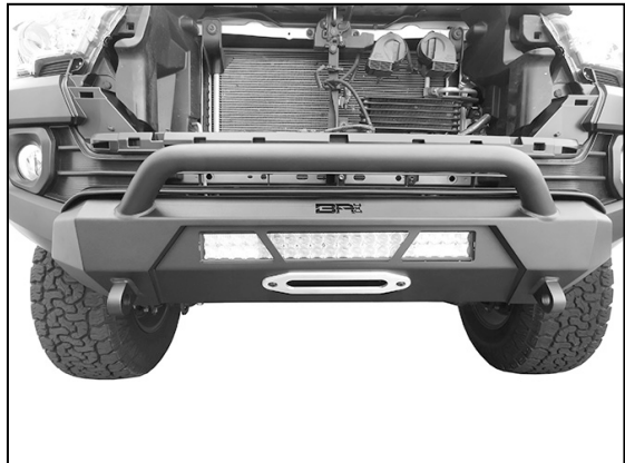
(Fig 33) Check fit of Bumper to plastic and trim as necessary. Reinstall grille and top cover
