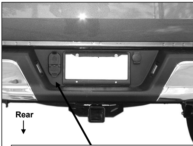
(Fig 1) Unplug and remove 7-wire trailer plug
