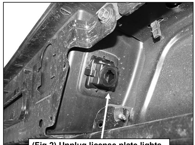
(Fig 2) Unplug license plate lights
