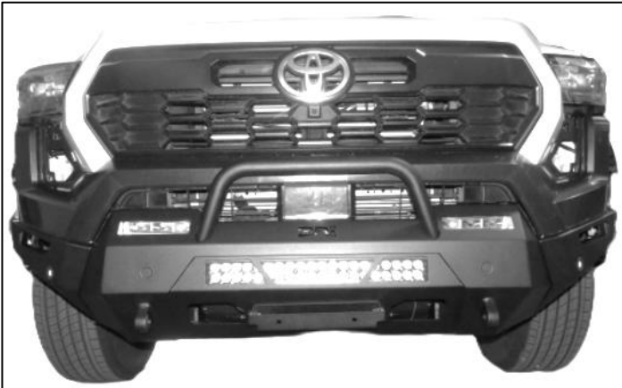
(Fig 36) Reattach and tighten all hardware for the Front Fascia. Make sure all clips go into their original latch points and wire harness is clear of any interference/pinching points.
