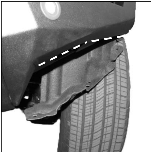
(Fig 40) Trim exposed section of the fender liner
