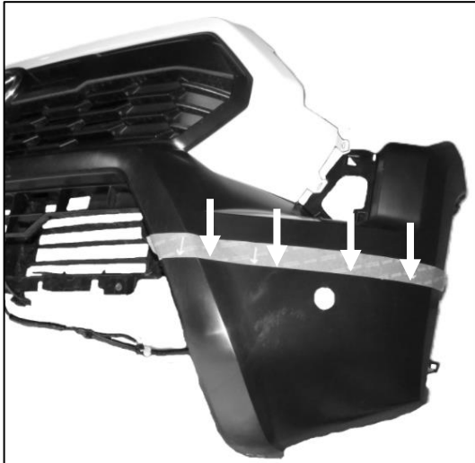
(Fig 18) Mark out the cut line, make sure any electrical components/harnesses are clear, and carefully cut the plastic.
