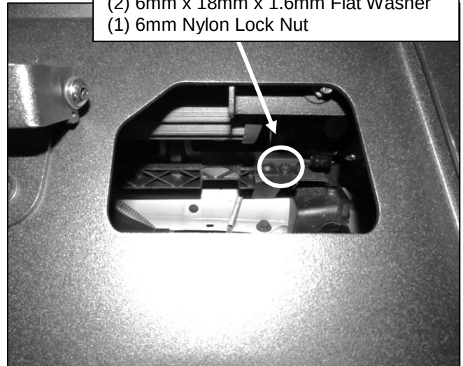
(Fig 37) Reach through the lower openings in the Bumper and secure the lower outer mount points of the active grille shutter assembly onto Upper Support Brackets using indicated hardware. It may also be helpful to reach behind the factory fascia through the wheel well. (Driver side shown)
