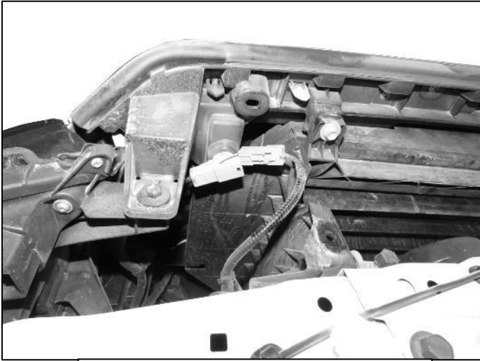
(Fig 11) Unplug driver side wire harnesses shown
