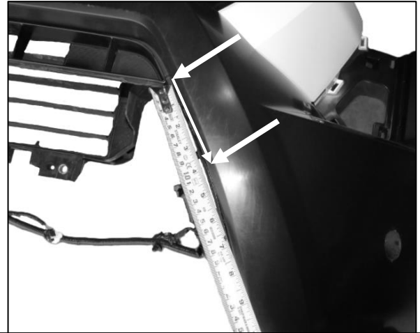
(Fig 15) Measure approximately 100mm/ 4in down from the corner from the factory grille insert.
