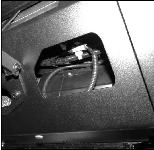
(Fig 7) Reach through the lower openings on each side of the Front Bumper Assembly and disconnect the fog lights and front parking sensors (if equipped).
