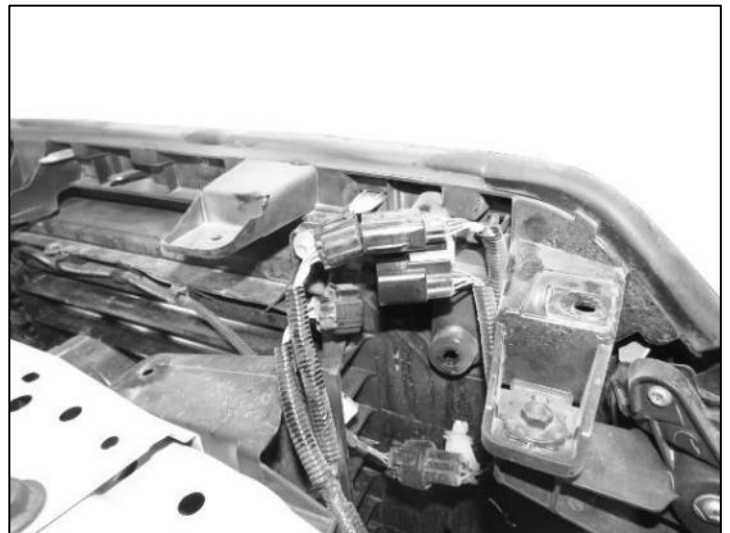
(Fig 10) Unplug passenger side wire harnesses shown
