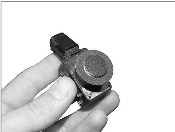
(Fig 24) Apply Adhesive Foam ring to end of sensors
