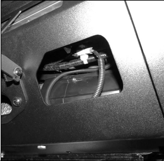
(Fig 38) Reach through the lower openings on each side of the Front Bumper Assembly and plug in the fog lights and bumper mounted parking sensors using the Parking Sensor Extension Harnesses (if equipped)
