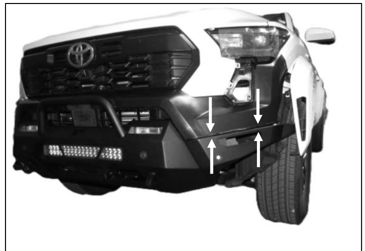
(Fig 33) Carefully reinstall the factory plastic front fascia onto the vehicle and check fitment between the Side Wings and the plastic fascia. Adjustments to the Side Wings or additional plastic trimming may be necessary. Do not fully tighten fascia hardware until adjustments/trimming are complete
