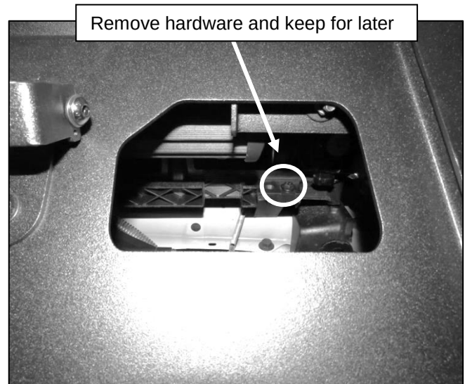
(Fig 6) Reach through the lower openings in the Bumper and remove the hardware that secures the lower outer mount points of the active grille shutter assembly onto the Upper Support Brackets. Keep this hardware as it will be reused to reinstall the front fascia. (Driver side shown)
