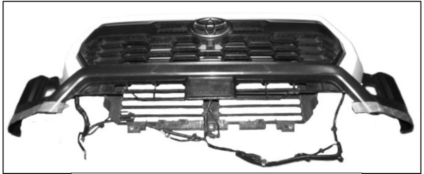
(Fig 19) Repeat the cutting procedure on the other side of the plastic fascia.
