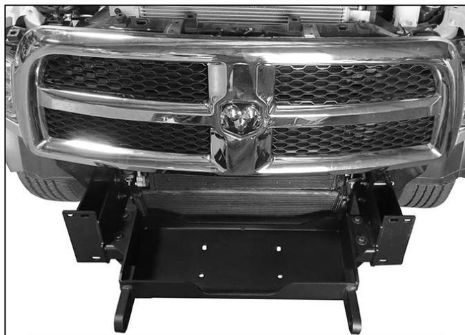
(Fig 10) Attach Winch Tray to Frame Brackets
