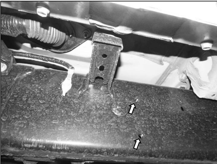
(Fig 5) On rear section of the frame, locate the rear threaded inserts
