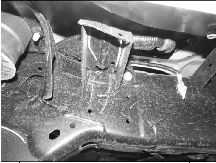
(Fig 7) On rear section of the frame, locate the rear threaded inserts
