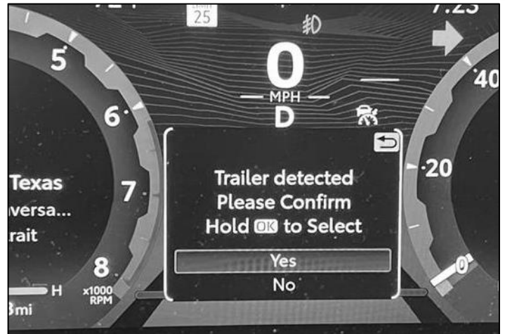
(Fig 21) Possible error warning if BSM not installed correctly
