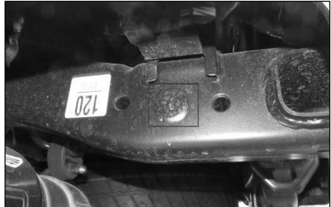
(Fig 25) Remove the center plastic caps on the outer side of the rear frame on both the DS and PS
