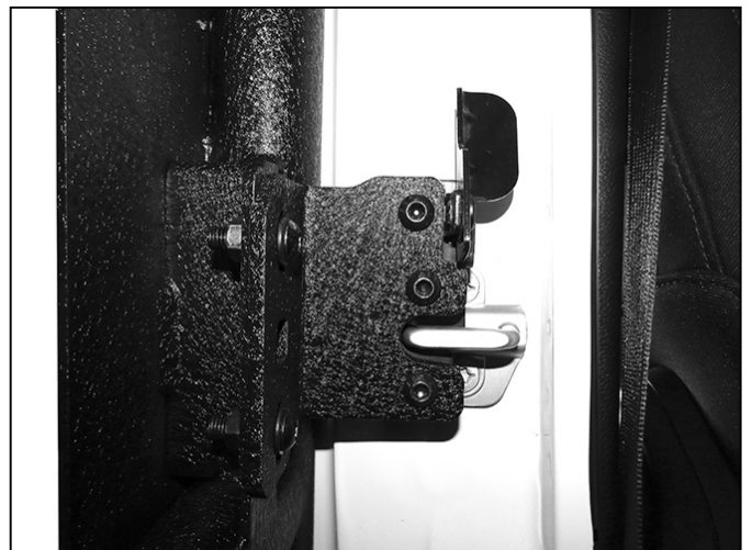
(Fig 15) Adjust Door and Latch assembly for proper operation before fully tightening hardware. Make sure door latch fully closes against striker
