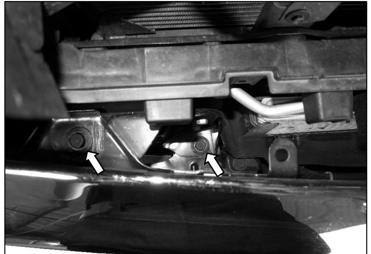
(Fig 10) On passenger side top of front bumper, remove bolts to detach bumper from frame of vehicle.
