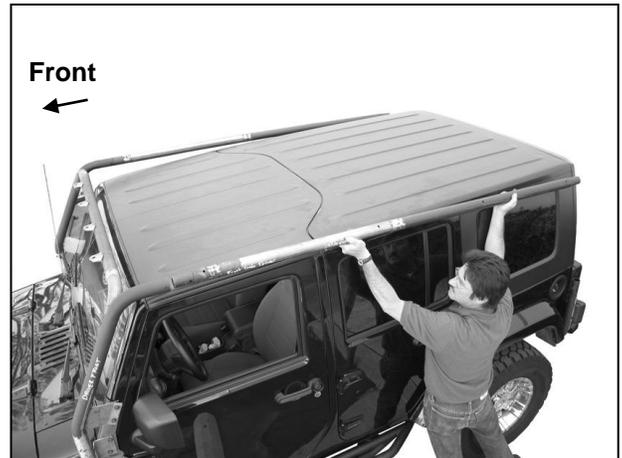
**(Step 7)** Move to the rear of the vehicle. Determine correct procedure to install the rear mounting legs. **IMPORTANT:** Models with factory or “wrap around” style bumper, drilling is required to attach short Rear Mounting Base to side of body. Skip to **Step 14**.
