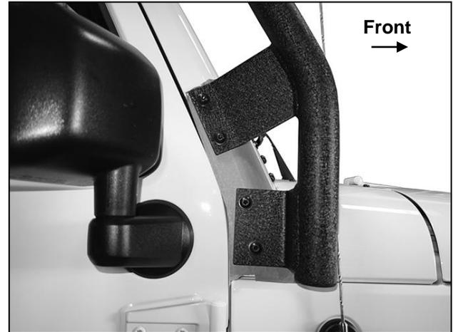
**(Step 4)** Select Front Main Cross Tube. Insert Cross Tube into passenger/right Front Rack Leg. **NOTE:** Cross Tube can be installed with light tabs to the front or rear.
