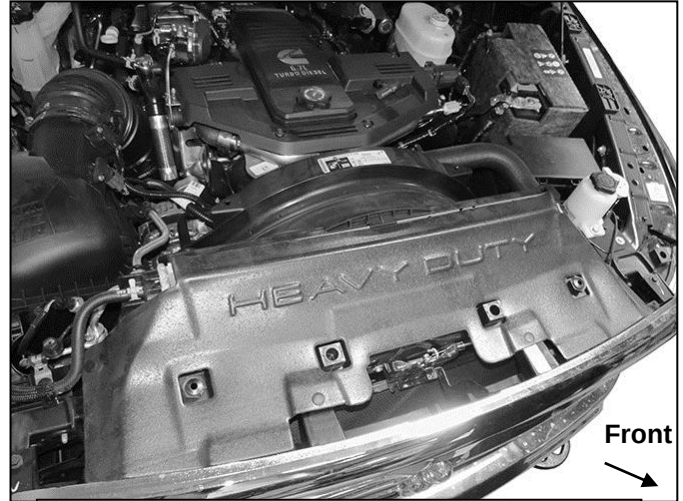
(Fig 2) Open hood and remove plastic cover
