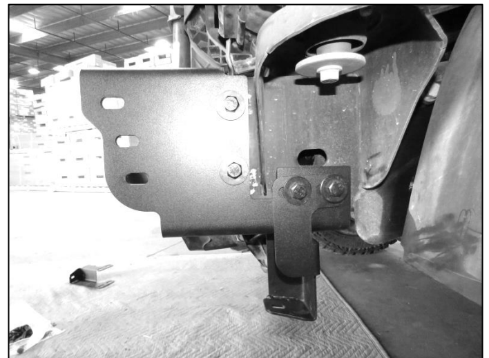
(Fig 10) Driver/left Skid Plate Support Bracket installed together with Frame Bracket
