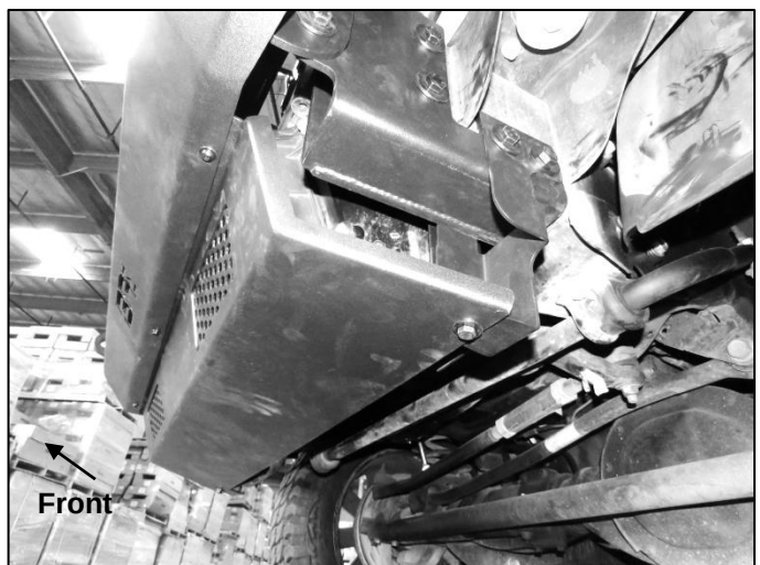
(Fig 21) Skid Plate installed
