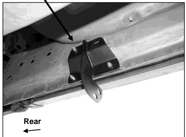
(Fig 8) Driver/left rear Bracket installed
