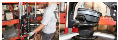
7) PLACE STRUT SPACER ON TOP OF THE STRUT AND TIGHTEN USING FACTORY HARDWARE.
