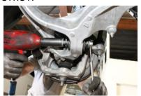
**4)** SUPPORT THE LOWER ARM WITH AN ADJUSTABLE JACK, MARK A REFERENCE LINE ON BOTH LOWER CONTROL ARM CAM BOLTS, THEN LOOSEN AND REMOVE BOTH BOLTS.
