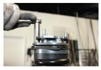
8) RE-INSTALL THE STRUT BACK INTO THE TRUCK USING PROVIDED NUTS ON TOP AND THE FACTORY BOLT ON THE BOTTOM, THEN ADJUST THE JACK UP SO THAT THE LOWER CONTROL ARM CAMS CAN BE RE-INSTALLED. ONCE INSTALLED, LINE UP YOUR MARKS AND TIGHTEN THE CAM BOLTS.
