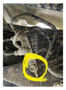
Hard brake lines bracket bolt must be removed to have room to slide the bracket with the double nuts plate.
