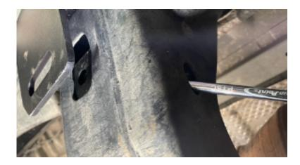
On this step, you will need to take your time and be patient to get the alignment properly. As stated before, you can add an optional small amount of thread locker to ensure the bolt does not backout.
