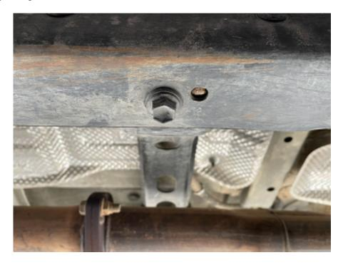
\*\*Please note on some frames there are plastic caps or stickers covering the holes where the bolts go through. If your truck has those, carefully remove them with a flat screwdriver or peel the stickers off from both sides of the truck. \*\*
