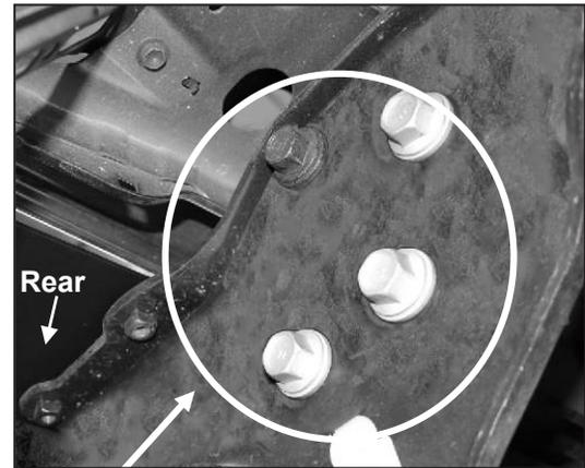
(Fig 2) Remove factory bolts attaching bumper assembly to frame
