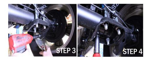
5. Use the floor jack to lift the rear axle, keeping the pin aligned with either the centered hole or the offset hole, and install the new u-bolts with the provided hardware. **NOTE: TORQUE U-BOLTS TO 100 FT/LBS**
