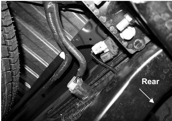
(Fig 1) Unplug and remove 7-wire trailer plug, unplug license plate lights and sensors if equipped
