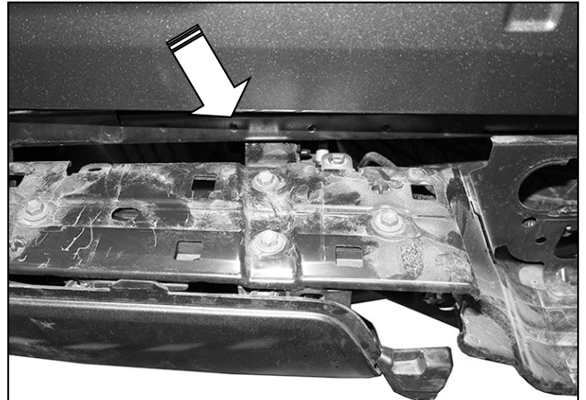
(Fig 5) Models with receiver hitch, remove the hex bolts attaching bumper to top of hitch
