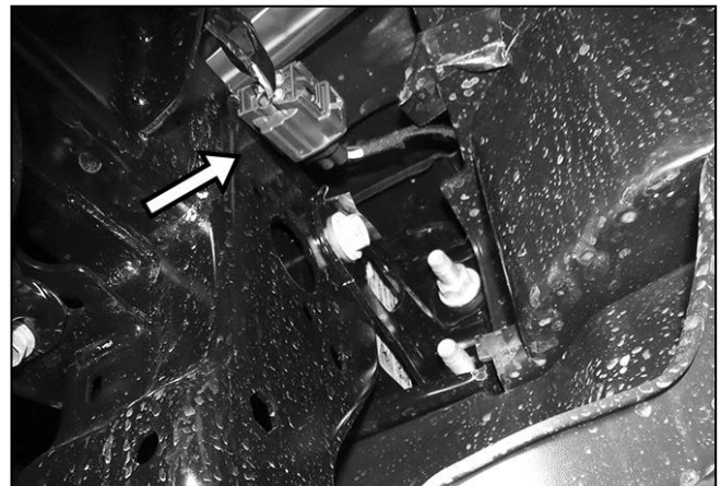
(Fig 2) Unplug the wiring harness leading to the front bumper (arrow-JL passenger side pictured)
