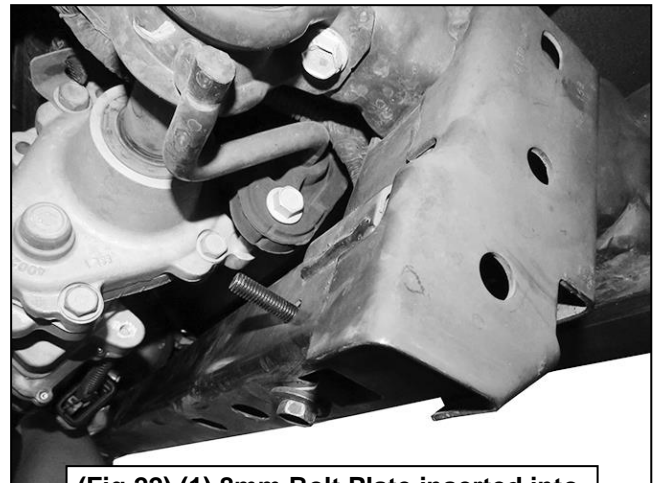
(Fig 22) (1) 8mm Bolt Plate inserted into the crossbar (Passenger/Right shown)
