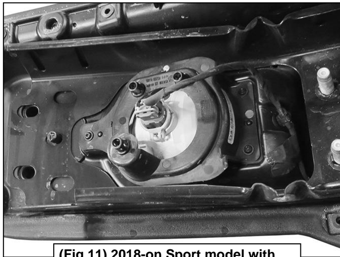
(Fig 10) Factory fog light attached to the back of the Bumper (4 pin fog light mounting shown)
