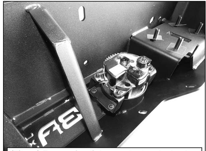
(Fig 10) Factory fog light attached to the back of the Bumper (4 pin fog light mounting shown)
