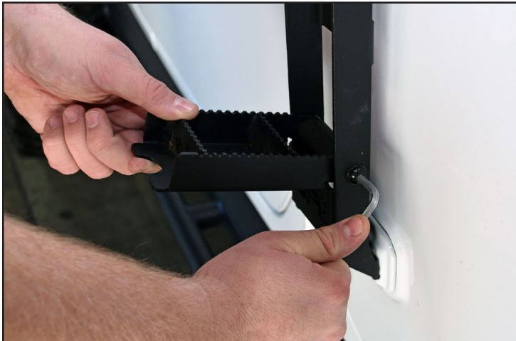
PIC 04: Adjust step pivot tension.
