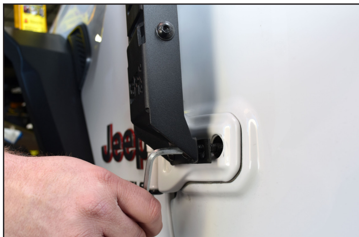
PIC 02: Install the Door Hinge Step.
