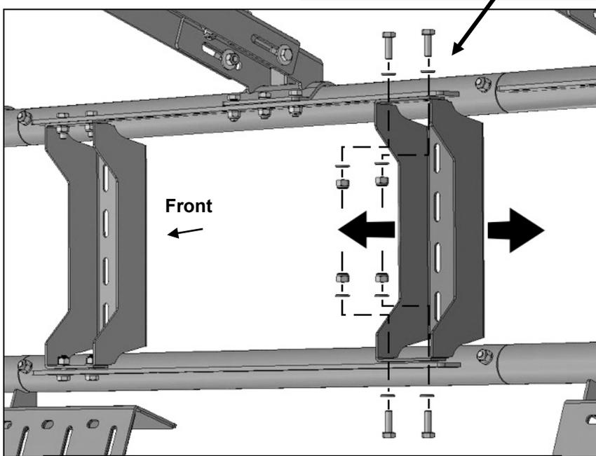
(Fig 1) Attach Accessory Bracket to mounting tracks on back of Side Tubes (passenger/right side illustrated)
