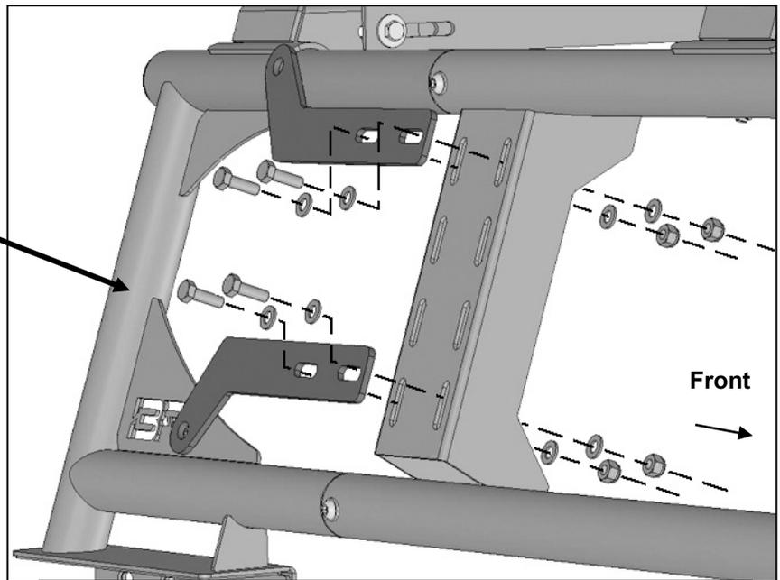
(Fig 2) Example of typical Universal "L" Bracket installation
