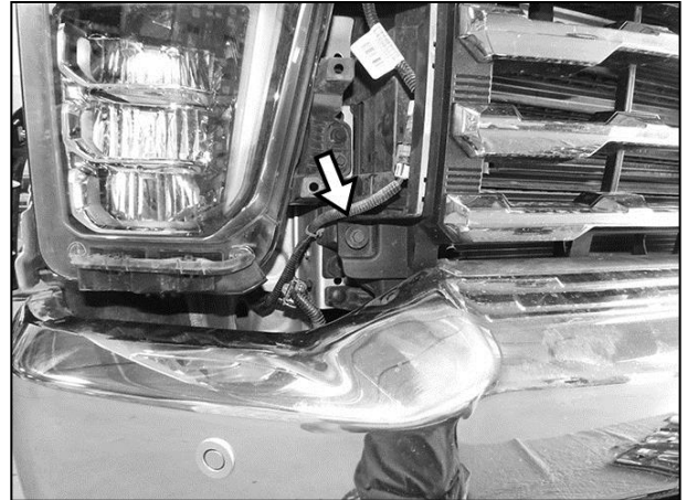
(Fig 6) Disconnect all wire harnesses leading to front bumper. Disconnect harness to camera (if equipped) and remove grille
