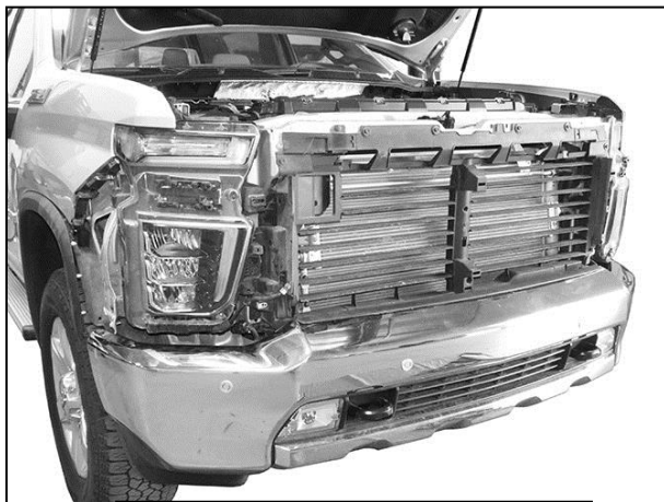
(Fig 7) Grille and fascia removed
