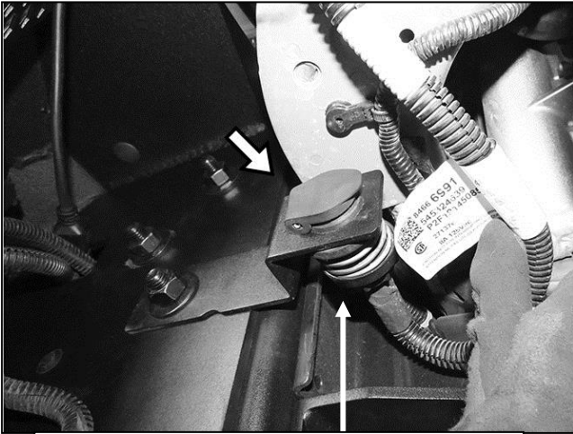
(Fig 31) Models with block heater, attach Relocation Bracket to outside of driver/left Mounting Bracket (arrow)
