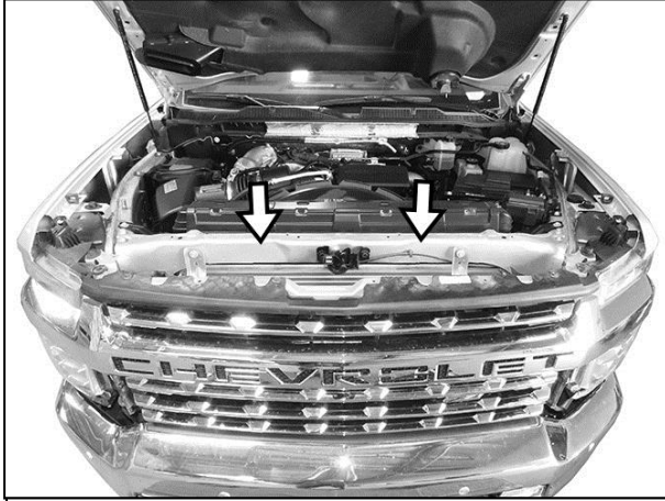
(Fig 5) Remove plastic cover from top of grille
