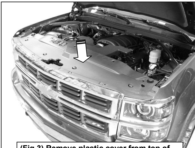
(Fig 3) Remove plastic cover from top of radiator (arrow). Temporarily remove grille
