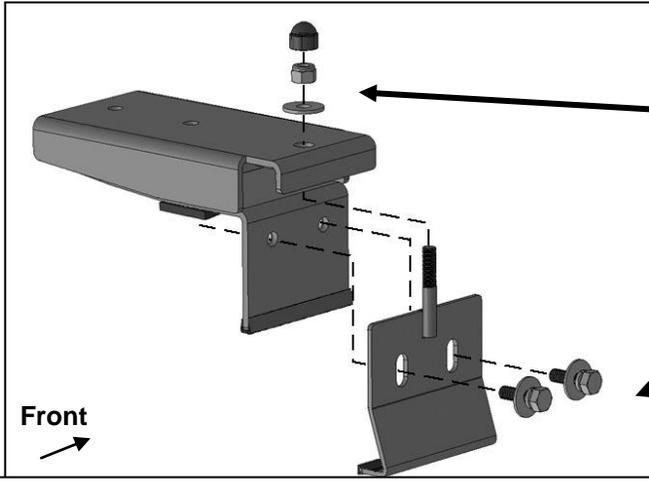
**Attach Clamp Bracket to Mounting Bracket:**
