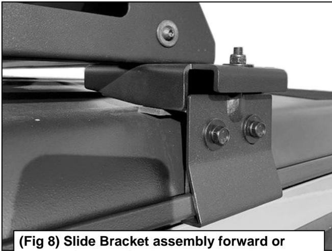
(Fig 8) Slide Bracket assembly forward or back to line up with Basket. Attach Basket to the Front Brackets (passenger/right pictured)
