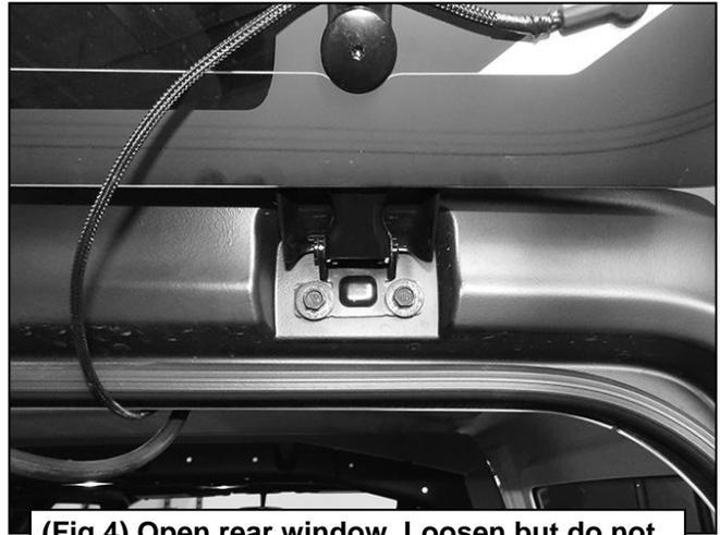
**(Fig 4) Open rear window. Loosen but do not remove (2) rear window hinge bolts (arrow)**
