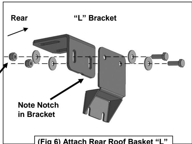
**(Fig 6) Attach Rear Roof Basket "L" Bracket to Rear Window Bracket**
