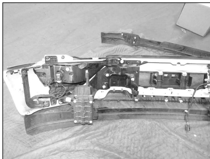
(Fig 17) Remove parking sensors and harness from factory bumper if equipped
