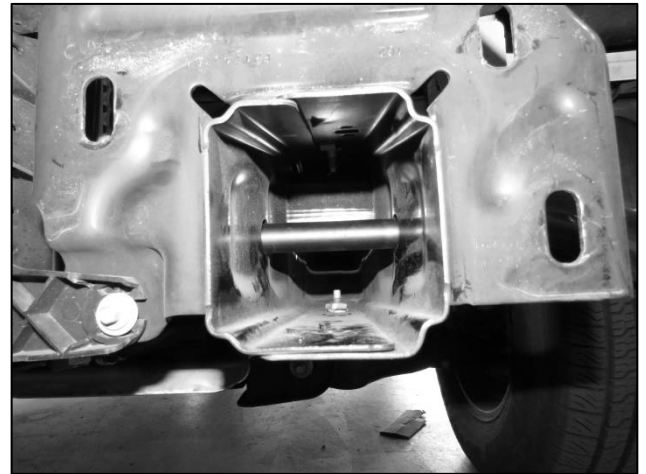
(Fig 9) Spacer tube installed inside of frame.
