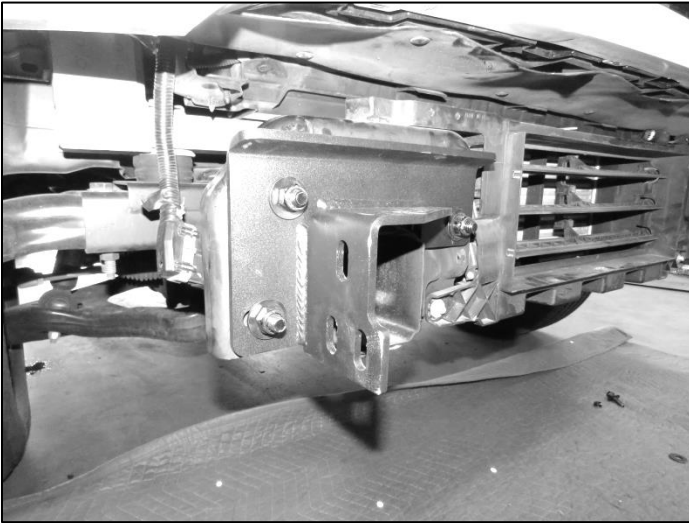
(Fig 12) Passenger/Right side bracket installed.
