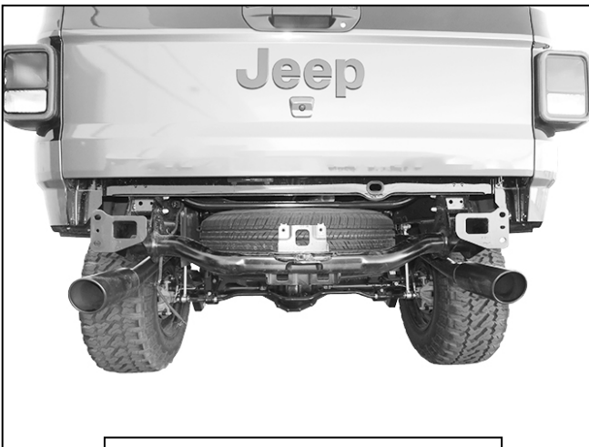
(Fig 8) Factory bumper removed
