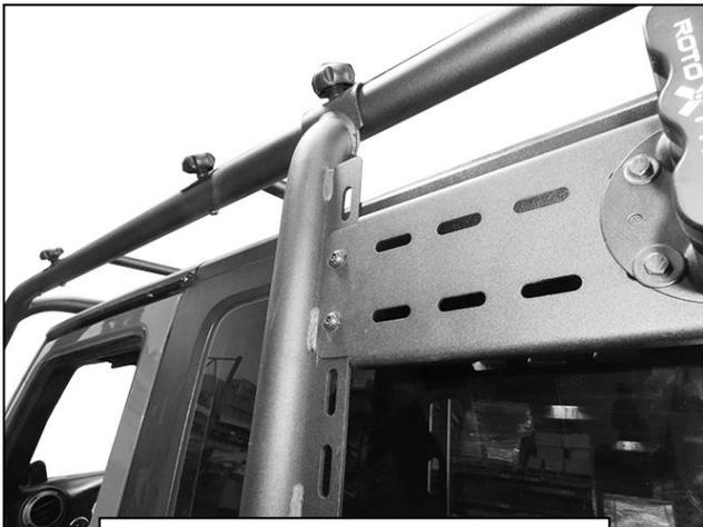
(Fig 10) Accessory Plate attached to the front Accessory Tube
