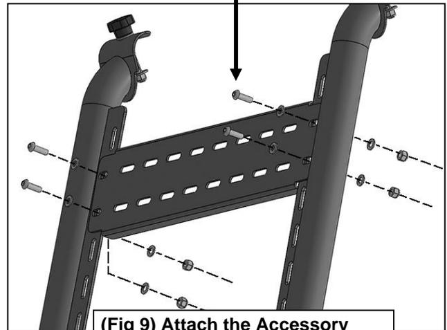
(Fig 9) Attach the Accessory Plate to the (2) Accessory Tubes
