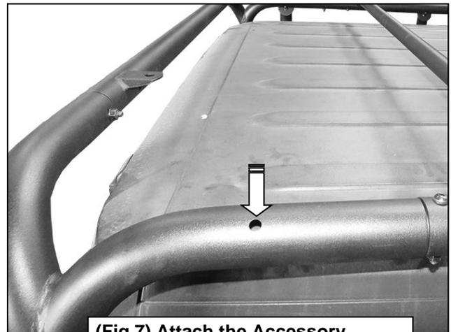
(Fig 7) Attach the Accessory Tubes to the holes in the roof rack, (Passenger/Right rear shown)
