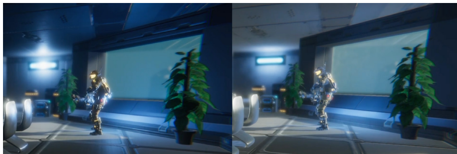
The effect of light baking on shadows: before baking on the left, and after baking on the right
