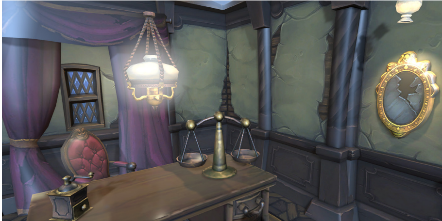
A shader is applied to a sphere-shaped Point light to provide a halo effect around it
