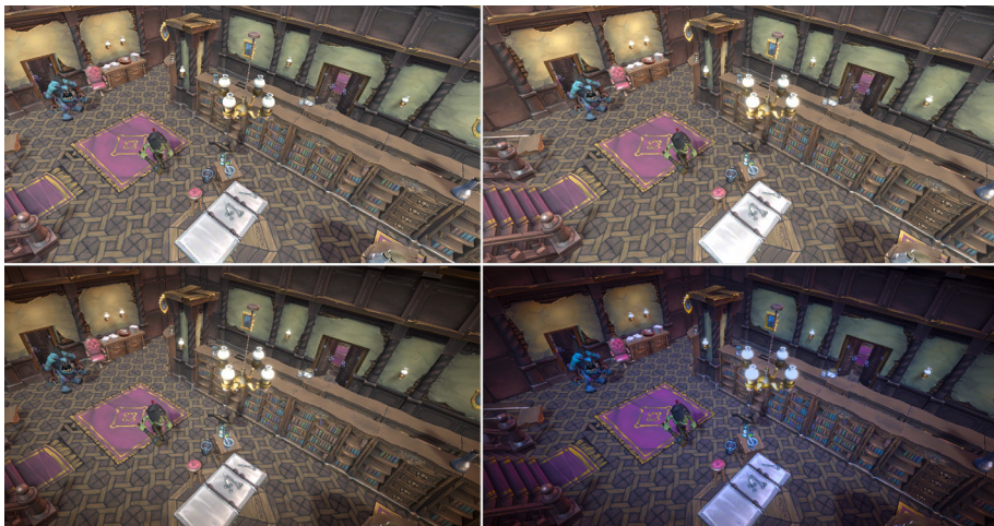
Applying post-processing effects: The top-left image has no effects applied, the top-right image has Bloom applied, the bottom-left has Vignette applied, and the bottom-right has Color Adjustment added.
