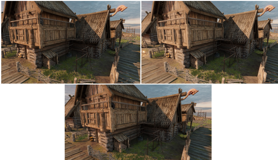
Comparing scenes rendered using different shaders: The top-left image uses the Lit Shader, the top-right, the Simple Lit Shader, and the bottom image, the Baked Lit Shader.
