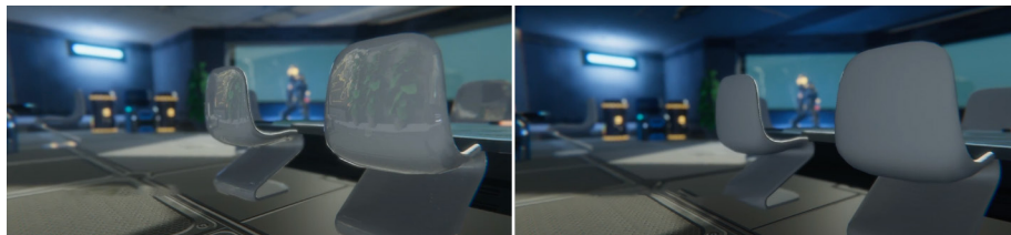
The effect of using Reflection Probes on smooth surfaces: with Reflection Probes on the left and without on the right
