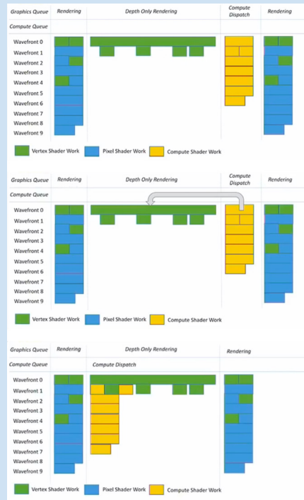
Async Compute can move compute shader work in parallel to the graphics queue.
