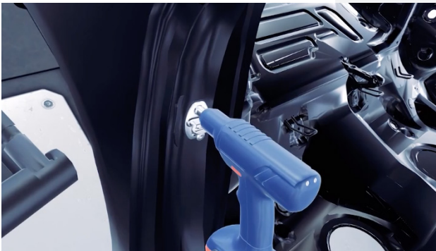
VR training for manufacturing employees – using a drill to fasten door bolts
