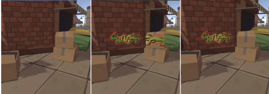
From left to right: No decal in the image, the decal hitting all objects, and the decal applied to the wall only, using Rendering Layers
