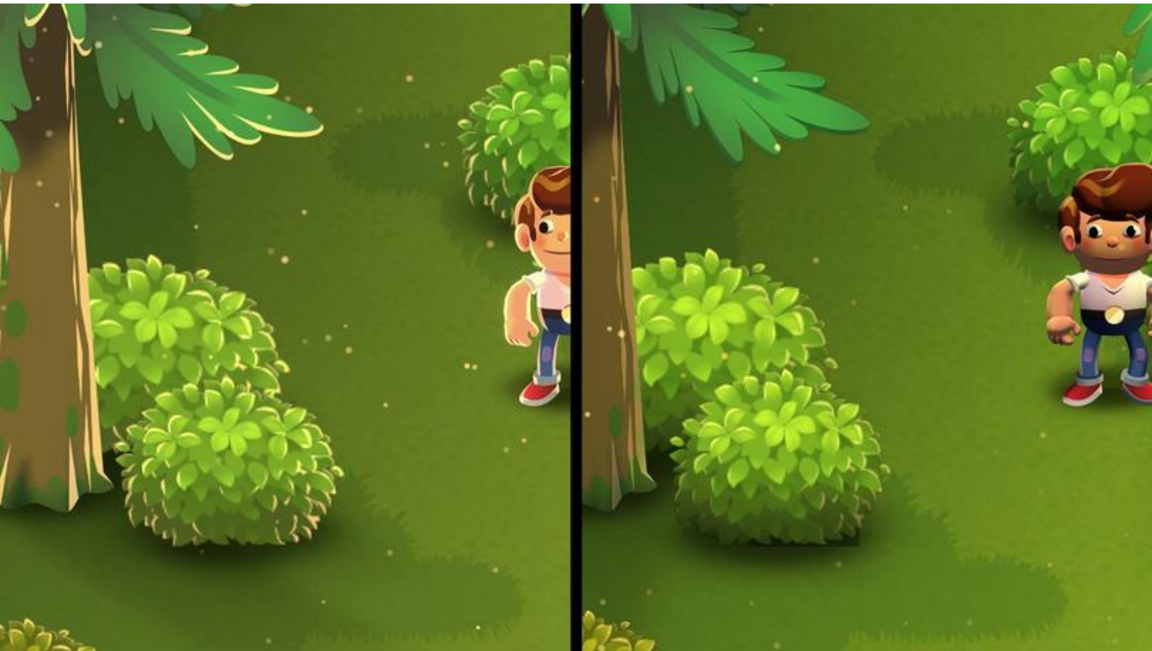
The bushes in Happy Harvest appear to have depth thanks to normal maps (enabled by the normal map option in the Light component).
