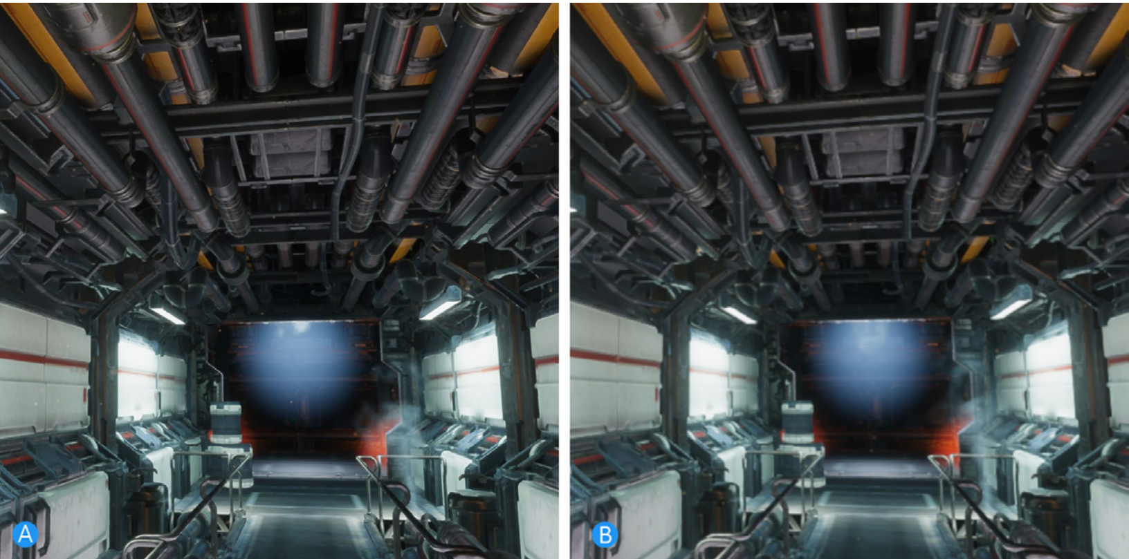
Image (A) to the left, using the Temporal Anti-Aliasing Upscale method, is sharp and well-defined. Image (B) to the right, which uses the Catmull-Rom upscale method, appears less-defined.
