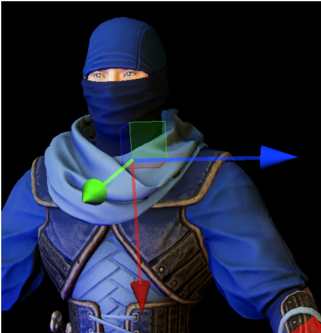
The head is using the Y positive for the Aim Axis and the negative X for the Up Axis.
