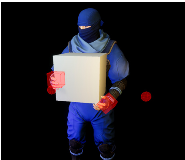
Two Bone IK constraints positioned to enable the character to carry a box
