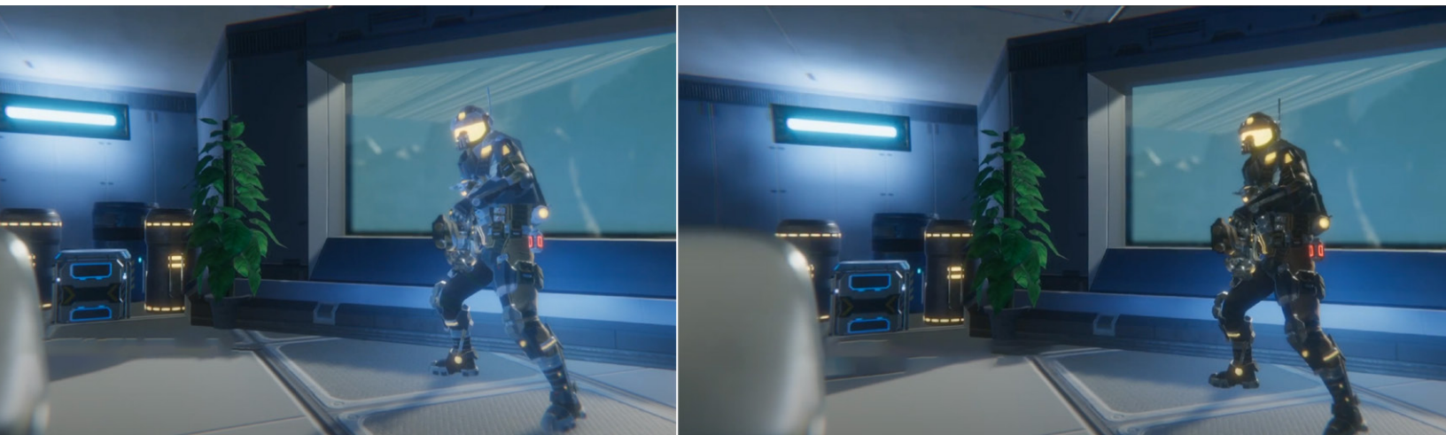
The effect of using Light Probes when rendering a dynamic object: with Light Probe on the left, and without on the right
