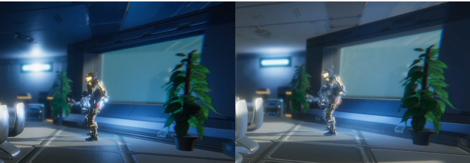
The effect of light baking on shadows: before baking on the left, and after baking on the right
