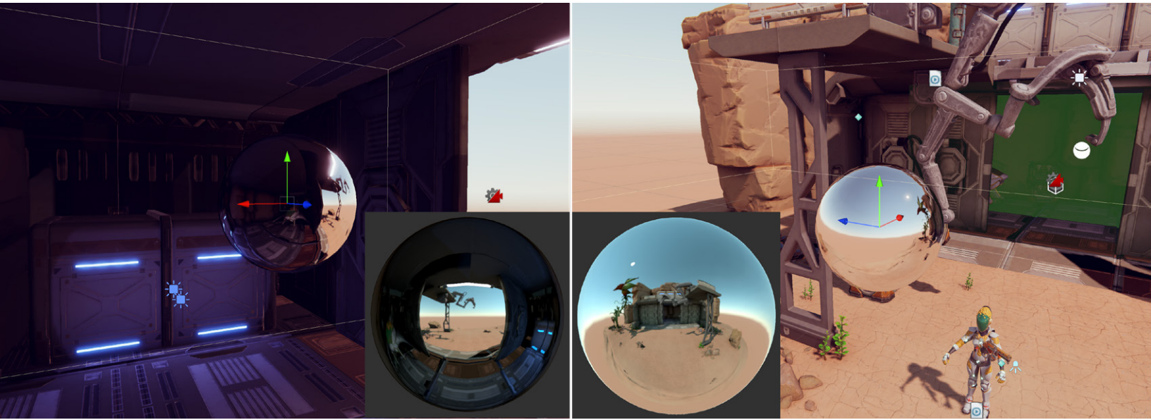
Each Reflection Probe captures an image of its surroundings in a cubemap texture.
