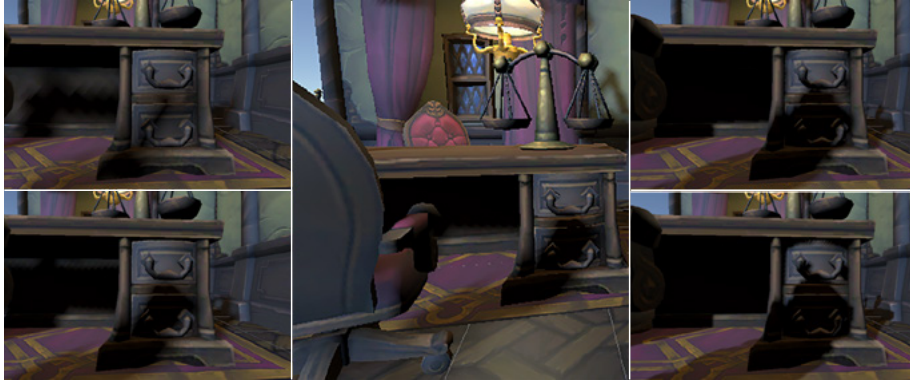
Setting the Shadow Resolution for the Main Light: The resolution is set to 256 in the top-left image, 1024 in the bottom-left image, 1024 in the top-right image, and 4096 in the bottom-right image. Middle image 1024
