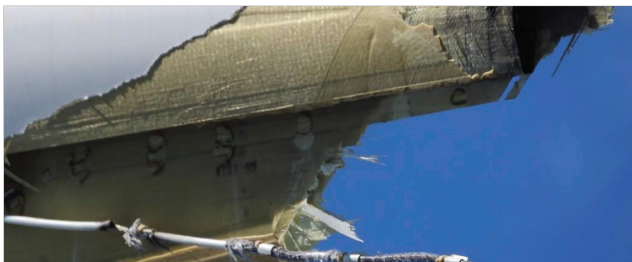
Fig 01 – Catastrophic lightning damage to blade
