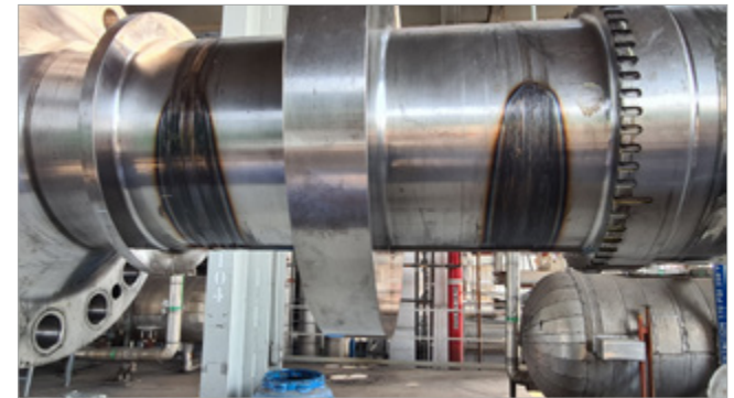
PHOTO: Severe damage to turbine shaft caused by lube oil system failure
