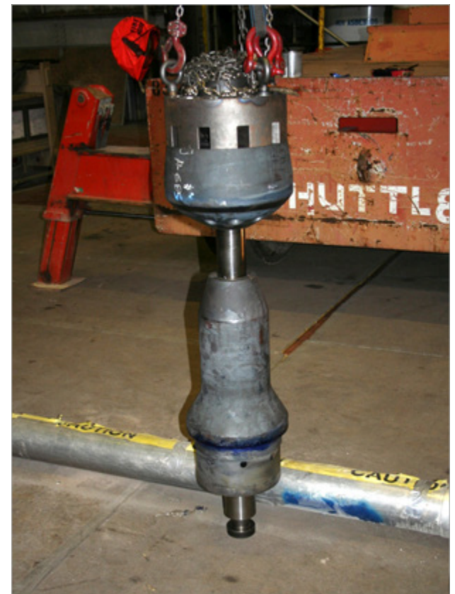
PHOTO: Valve cartridge for a steam turbine shutoff valve
