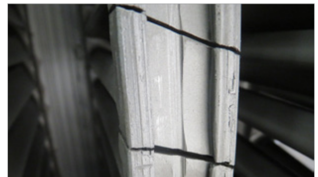
PHOTO: Damage to turbine blade tips due to severe misalignment and rubbing
