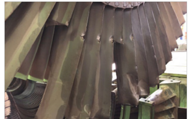
PHOTO: Result of a catastrophic overspeed
