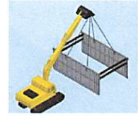
STAND TRENCH SHIELD IN UPRIGHT POSITION AND PREPARE FOR INSTALLATION
