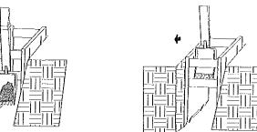
3. Pull shield forward by front spreaders or pulling eyes. Continue excavating and pull shield forward. Back fill as work progresses.
