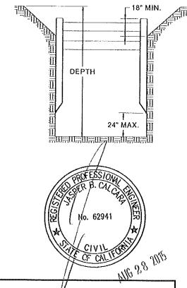
2" DIAM. PINS \$HALL HAVE MIN Fu = 92 KSI. CONTRACTOR RESPONSIBLE FOR ENSURING PROPER GRADE PINS ARE IN PLACE PRIOR TO SHIELD USE.
