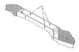
6. WARNING: Lift eyes are designed and intended for assembly and lifting only. Do not pull or lift by eyes when shield is stuck or has pressure against it. Loosen shield by pulling on spreader or digging along sides before using lift eyes.
