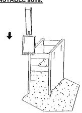
2. Continue excavating with in shield while alternately pushing down on shield corners, until proper grade is reached.
